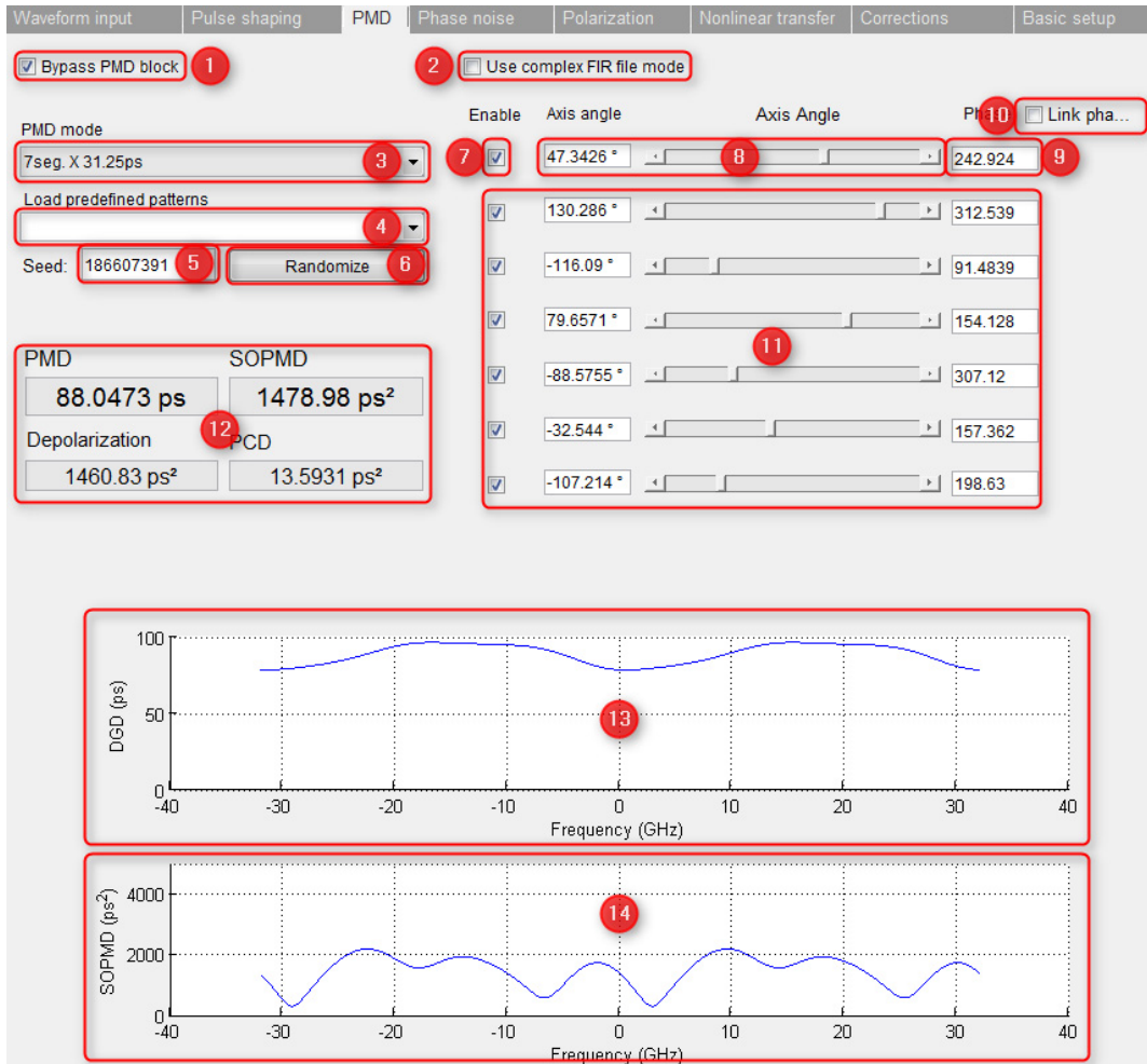
Figure 30 PMD tab (Concatenation of birefringent segments)
